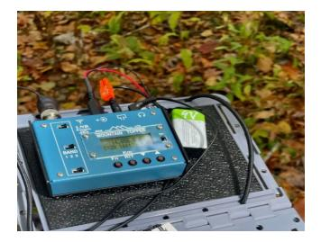
I love <u>these 9V rechargeable batteries</u>. It's hard to believe that the MTR-3B can complete 2-3 typically SOTA activations on one charge! Then again, the MTR-3B uses something like 18ma in receive? That's crazy low current consumption. These batteries are super lightweight and the particular brand I use has never produced any RFI (I've read that some others can). What's best is that I can recharge these easy via a USB-C cable.
